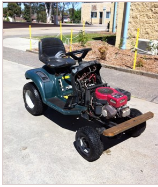
Tractor (ex ride on mower) LT X 16 Powered by 14.5 HP Briggs and Stratton
