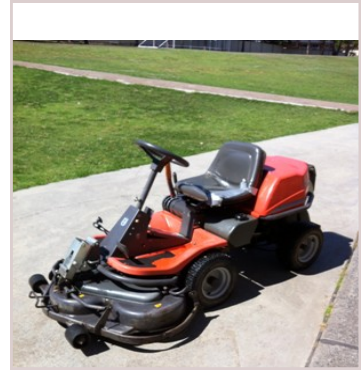
Husqvarna Ride-on Lawn Mower Rider Pro 15 Powered by 15 HP Kawasaki Hydra static 3 Cutting discs
